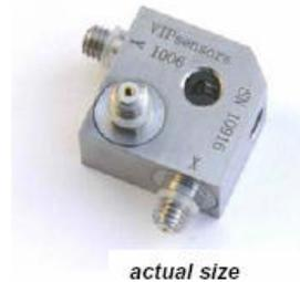
The Sensors Model 141 is a small triaxial piezoelectric accelerometer designed for vibration measurement in three orthogonal axes. Its light weight (17 grams) minimizes mass loading. The accelerometer is a self-generating device that requires no external power source for operation. The transducer features three M5 receptacles for output connection and is typically screw mounted.
